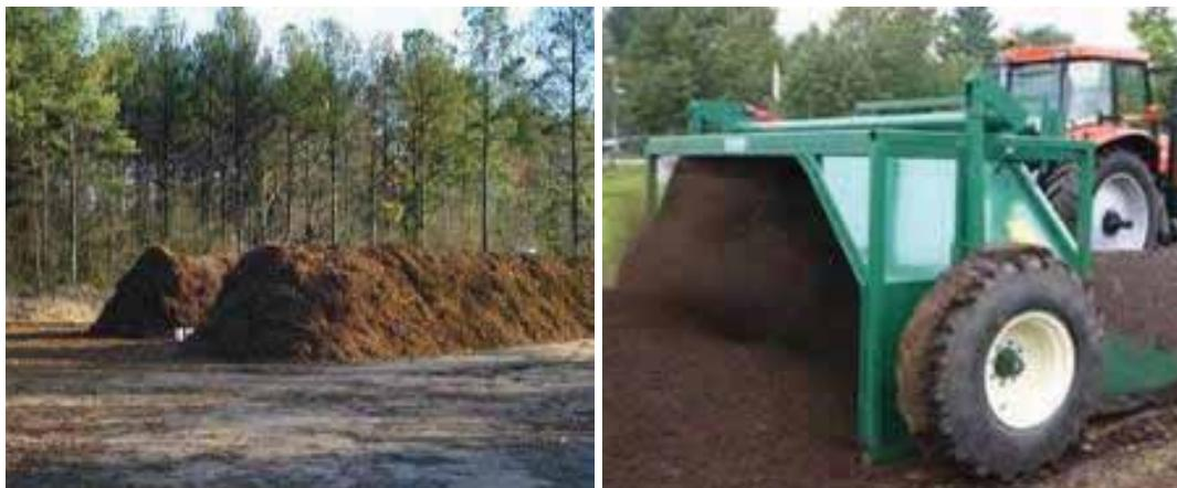
**Figure 10: Various auxiliary equipments are normally used, e.g. grinders, rotating screens, mixers, windrow turners and front-end loaders**
